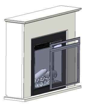
**Mounting Glass frame-** See Fig to the left. Product comes with a glass frame that is not fixed to firebox, but packed separately to the fire in its own packing.
