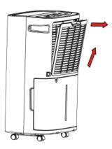
2. To clean, use a vacuum cleaner to gently absorb any dust accumulation on the filter screen surface. If there is a lot of dust, use warm water and a touch of detergent. Ensure to keep dry.
