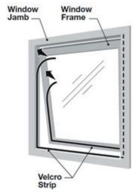
**Step 2:** Attach the window seal to the Velcro tape; ensure that there is no gap for the air to escape between the window frame and the window seal. The zip opening on the window seal must be located where the extendable hose outlet from the air conditioner can easily reach it. Open the zip to allow the outlet to be fitted and then close it tightly to hold the outlet in place.
