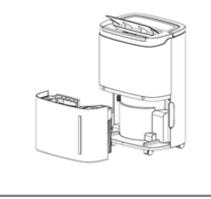
If using frequesntly, please clean the filter and the frame at least once every two weeks with cold or warm water, do not use chemical solvents or hot water.
