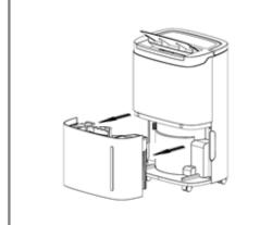
Close the tank cover and rotating water tank handle down, then put the water tank gently and put it back in the right place to restart dehumidifier.
