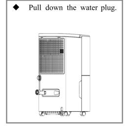
Connect a drainage pipe at proper length onto the water outlet.
