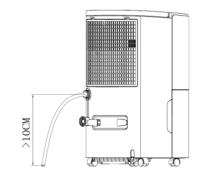
**Attention:** the level height of externally connected water pipe shall not be higher than the water outlet, and the water pipe at rear-end shall transit smoothly, otherwise, the leakage risk exists since drainage is not smooth.
