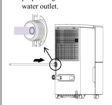
♦ Before using please check whether the drainage pipe is connected firmly or not in case that water leaks.
