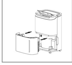
Attention: when the water tank is full of water, please empty it. Before putting the water tank into the dehumidifier, please confirm whether the floater rotates flexibly or not, and then push it in position with both hands.
