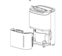
If using frequesntly, please clean the filter and the frame at least once every two weeks with cold or warm water, do not use chemical solvents or hot water.
